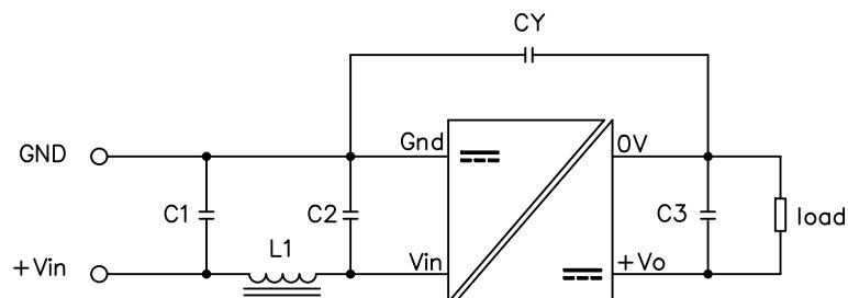
$C1/C2=4.7\mu F/50V$ ;  $C3=10\mu F/50V$  ; $CY =270pF/3KV$  ; $L1=6.8\mu H$
